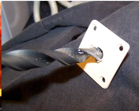
Fig. 5 Open up the jack plate so that the new jack will fit through it.
