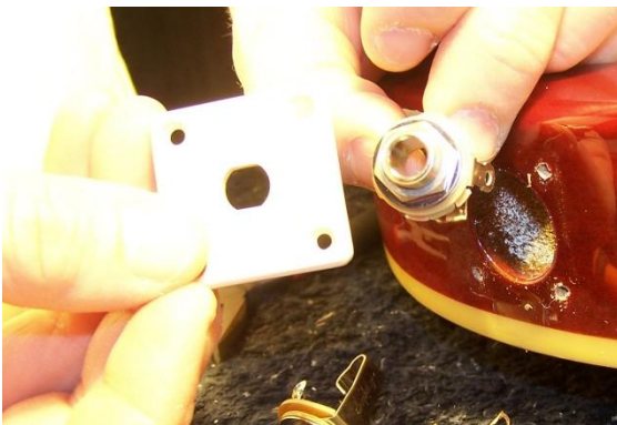
Fig. 5 Open up the jack plate so that the new jack will fit through it.
